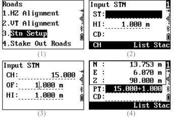
Press **F1[CH]** PIC(2) to set-up station by chainage. Input the chainage number and make sure that the inputted chainage is in the designed horizontal alignment PIC(3).
