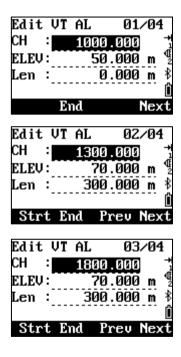
Input vertical curve data from computer through point and stake number, the vertical curve data should include the height, curve length, the curve length of start point and terminal point is zero.
